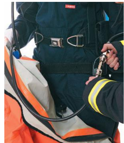
Connection of the air line with the SCBA inside of the suit
