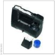
For retaining possible SO3, which can occur during measurement with Short-term Tubes.
