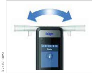
Mouthpiece receptacle can be mounted on left or right
